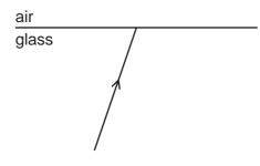
What happens if the angle of incidence is made larger than the critical angle for the glass?
